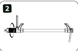
2. Fully loosen nut by turning counterclockwise.
