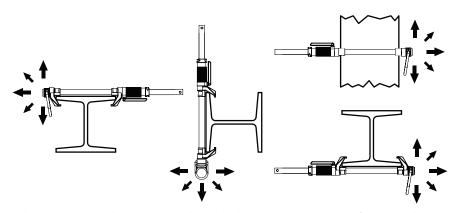
\*Note: Placement at or below a user's working height requires integration of a compatible ANSI Z359.1 shock-absorbing lanyard that does not allow user to extend more than 6 feet (2m) (in any direction) from the anchorage connector before shock absorber is activated. Beam anchor must be attached to I-beam flange facing the user (top flange if above, bottom flange if below, etc.).
